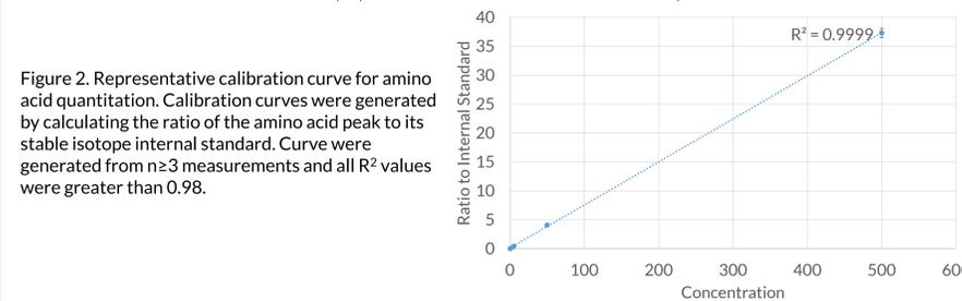
Figure 2. Representative calibration curve for amino acid quantitation. Calibration curves were generated by calculating the ratio of the amino acid peak to its stable isotope internal standard. Curve were generated from n≥3 measurements and all R<sup>2</sup> values were greater than 0.98.
