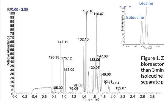
Figure 1. ZipChip separation of the t<sub>0</sub> timepoint from the bioreactor. The amino acids migrate through the chip in less than 3 minutes. As shown in the inset, isomers such as isoleucine and leucine are resolved and detected as separate peaks for confident identification and quantitation.
