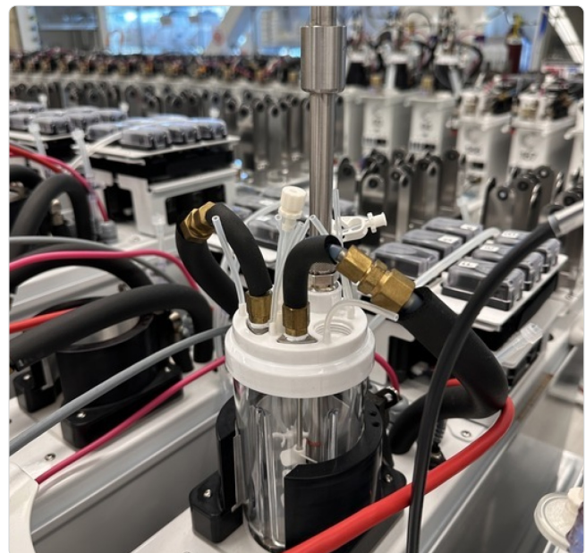
View of Culture Biosciences Cloud Bioreactor Lab with two reactors (288 and 289) setup with 908 Devices' MAVERICK device (left). Zoomed in view of the in-line probe inserted in a 250 mL vessel (right).
