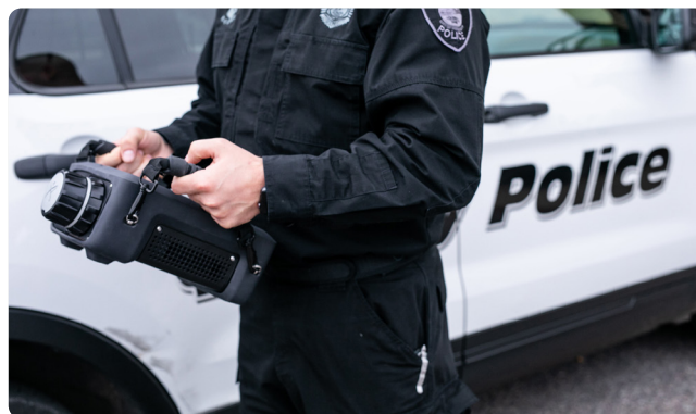
An officer operates a handheld mass spectrometry device with trace analytics directly in the field. Devices like this are used by Customs organizations around the world, including the New Zealand Customs Service. © 908 Devices
