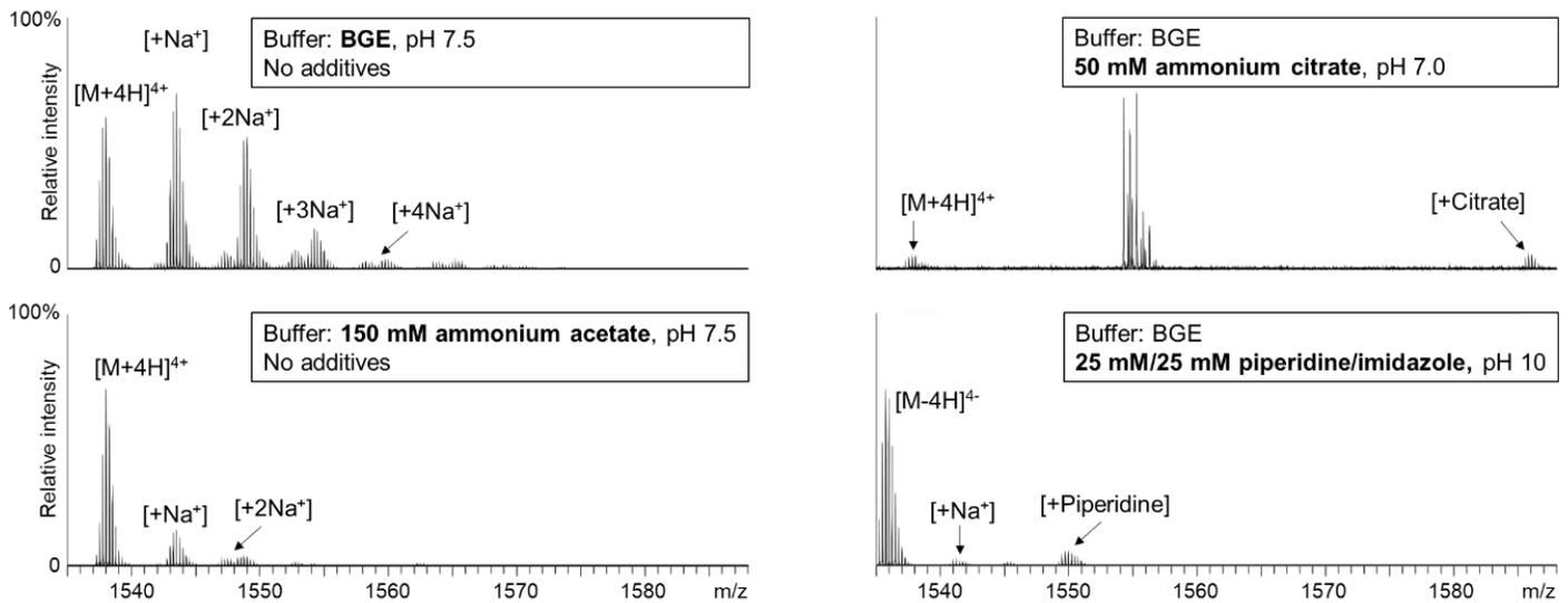
Figure 7: Static nanoESI mass spectra of the DNA 20mer standard collected on FT-ICR in either positive or negative ion mode. Only one charge state is shown to highlight the effects of the various conditions on the extent of salt adduction. The buffers and additives explored here were selected for their reported ability to reduce cation adduction.
