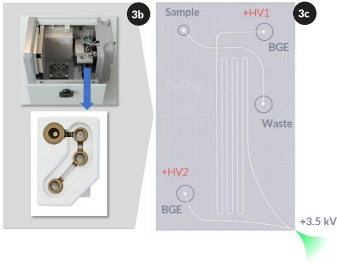
Figure 3. Factors affecting electrophoretic mobility of ions in CZE (a); ZipChip interface and microfluidic device (b); schematic of the microfluidic device (c).
