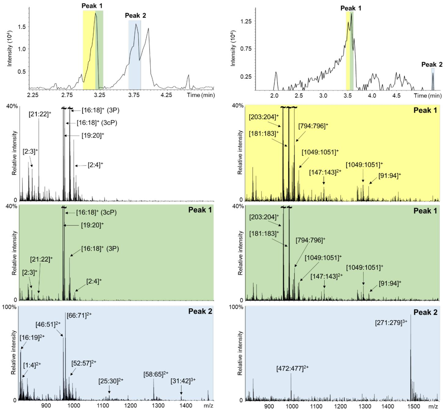
Figure 5: Electropherograms (top panels) and representative mass spectra of tRNA<sup>Phe</sup> (left column) and 18S rRNA (right column) digests. All data were acquired on timsTOF. 55 products out of 190 predicted hydrolytic products were detected for tRNA<sup>Phe</sup>, whereas 290 out of 525 for 18S rRNA.
