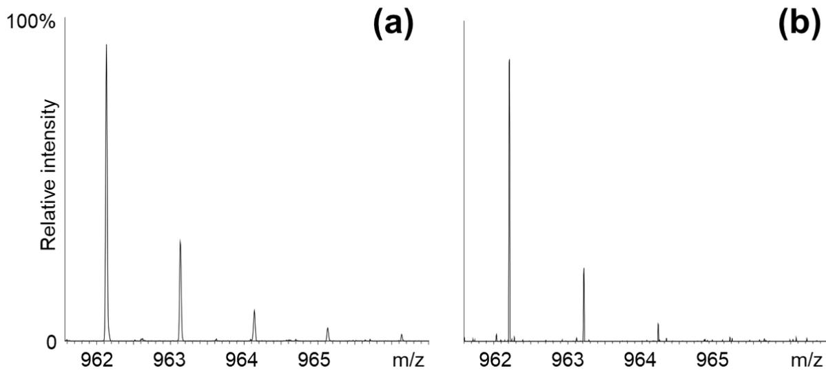
Figure 6: The performance of the mass analyzer can further affect the quality of the acquired data. Notice the ~40,000 vs. 70,000 resolution afforded by a) timsTOF vs b) FT-ICR determinations on the analysis of the [16:18](3P) digestion product. Both spectra were acquired in separation mode with ZipChip
