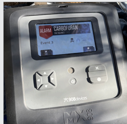
The MX908 can detect and identify 8 pesticides including Carbofuran, which the EPA has made ineligible for all uses.
