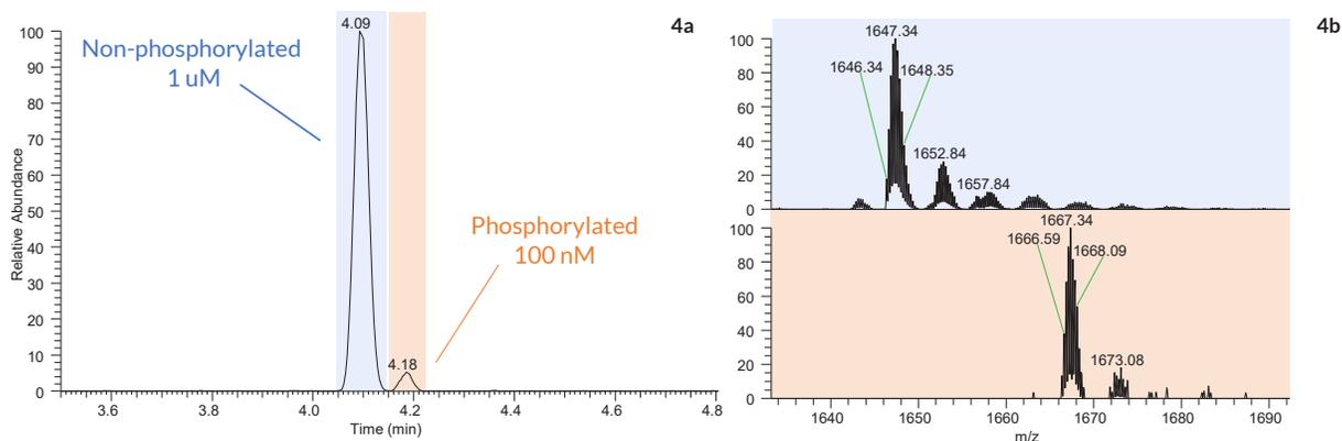
**Figure 4. Baseline resolved separation of phosphorylated RNA from the corresponding non-phosphorylated RNA standard**
