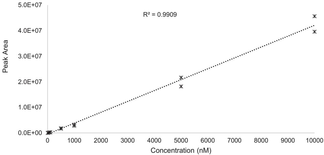
Figure 6. Calibration Curve showing good linearity and dynamic range for the unmodified 20 mer ssRNA standard
