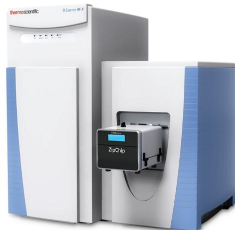
ZipChip mounted to a Thermo Scientific™ Q Exactive HF-X mass spectrometer.
