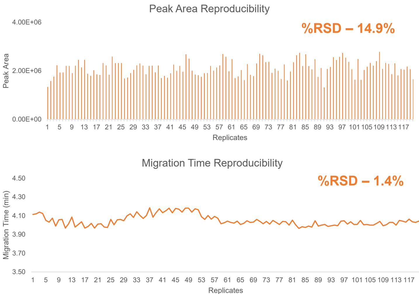
Figure 5. Replicate injections showing peak area (top) and migration time (bottom) reproducibility
