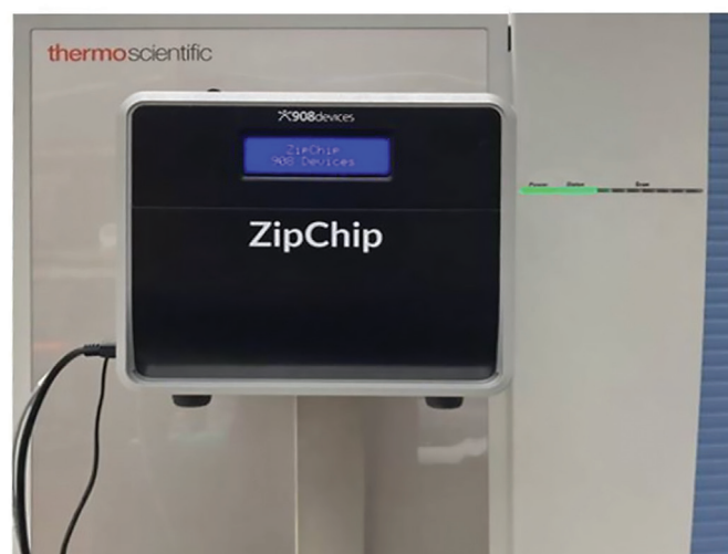
ZipChip mounted to a Thermo Scientific™ Orbitrap 240 mass spectrometer.
