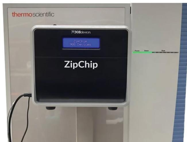
ZipChip mounted to a Thermo Scientific Orbitrap mass spectrometer.
