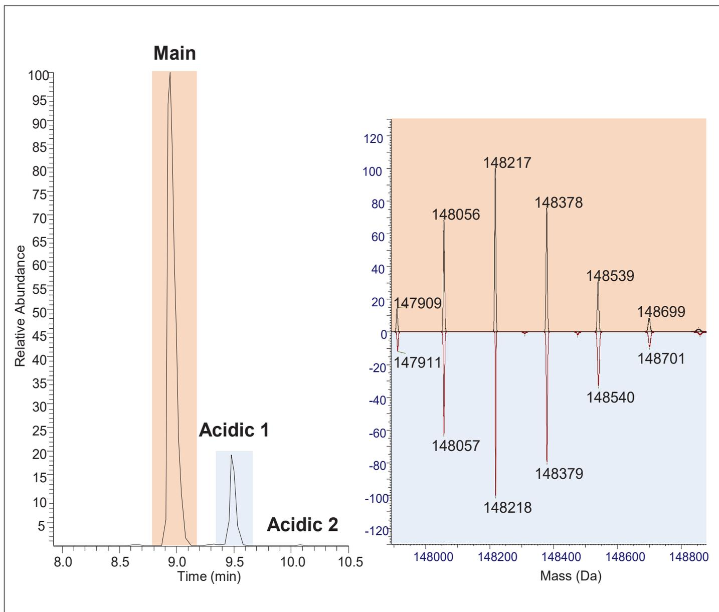
**Figure 3: Base peak electropherogram showing charge variants for trastuzumab (left) and comparison of the deconvoluted mass spectra of the main variant and acidic variant 1 (right)**
