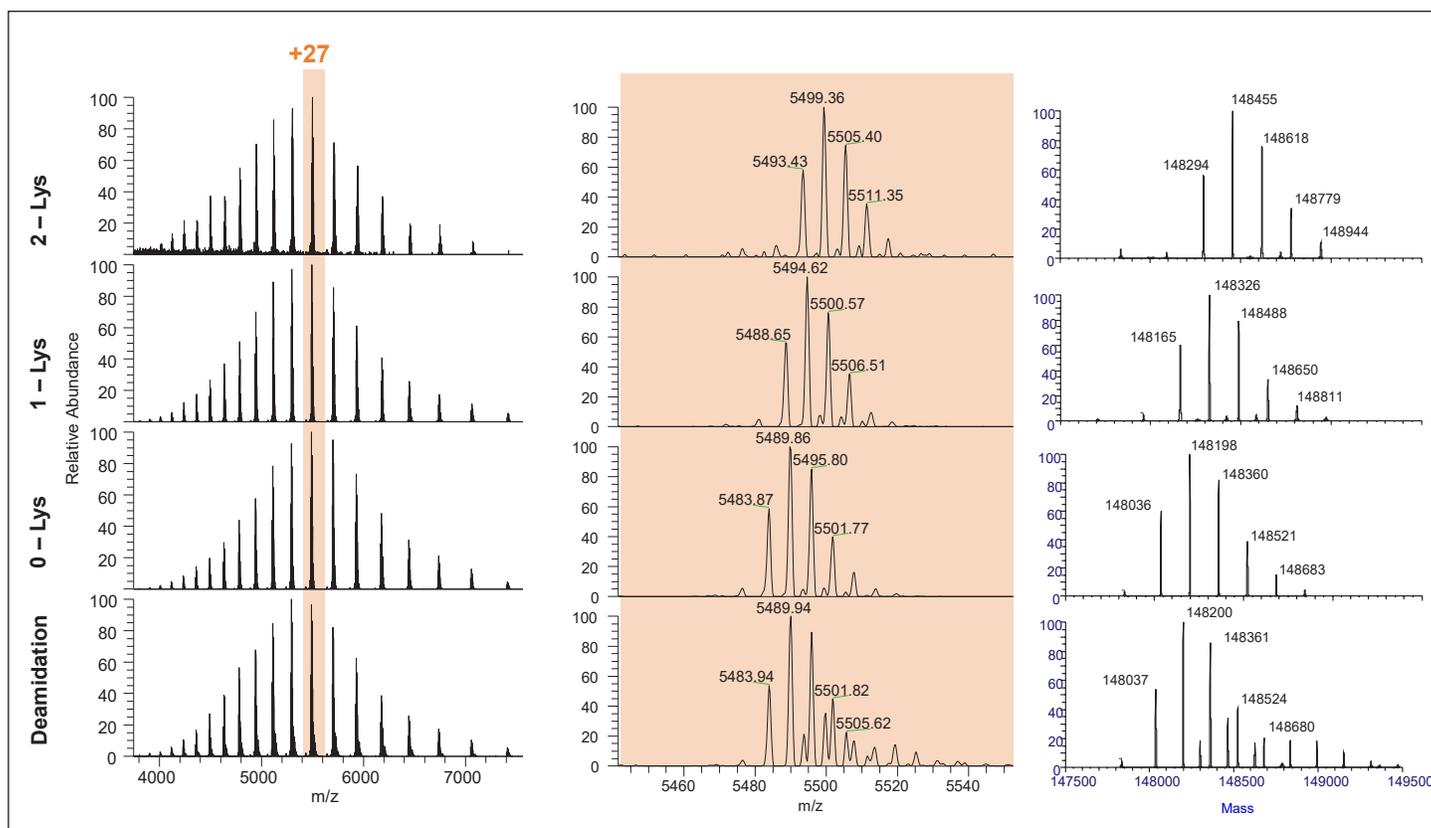
**Figure 2: Raw mass spectra for NISTmAb charge variants (left), zoomed-in spectra showing prominent charge state (+27) for charge variants (middle) and deconvoluted mass spectra (right).**
