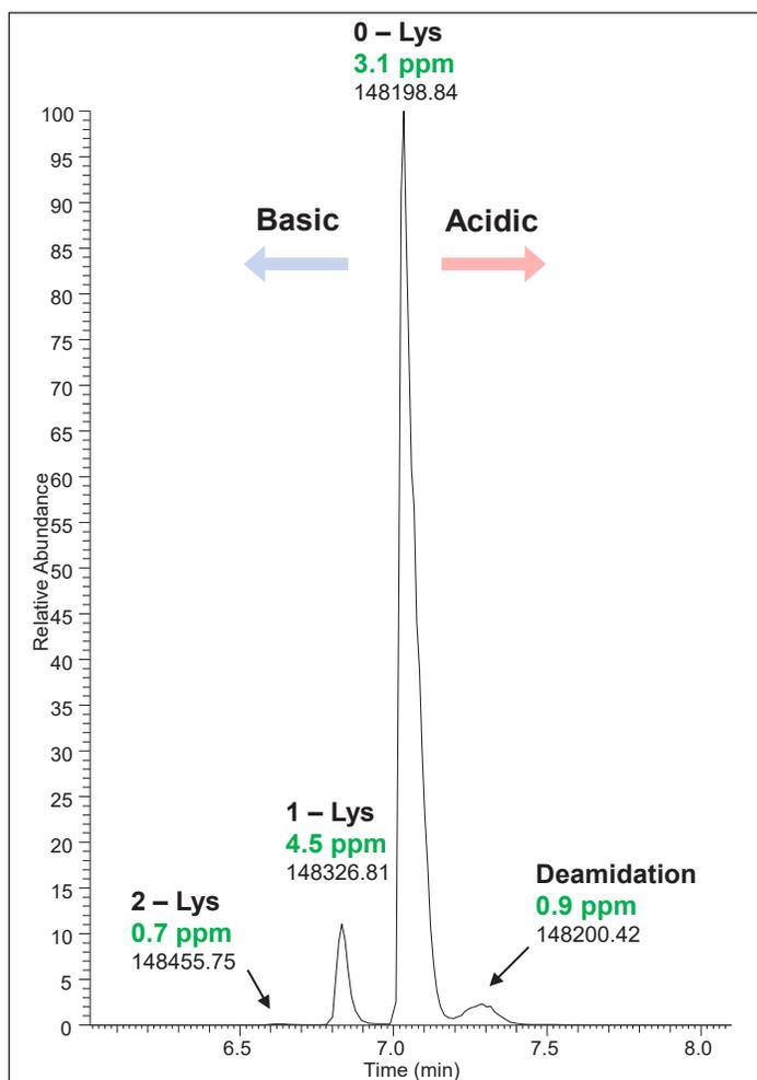
**Figure 1: Base peak electropherogram showing NISTmAb charge variants**
