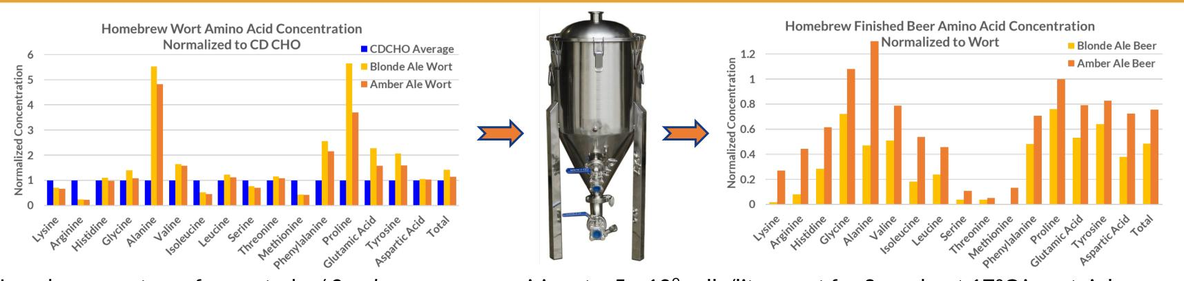
Homebrew wort was fermented w/ Saccharomyces cerevisiae at ~ 5 x 10<sup>9</sup> cells/liter wort for 3 weeks at 17°C in a stainless steel conical fermentation vessel.
